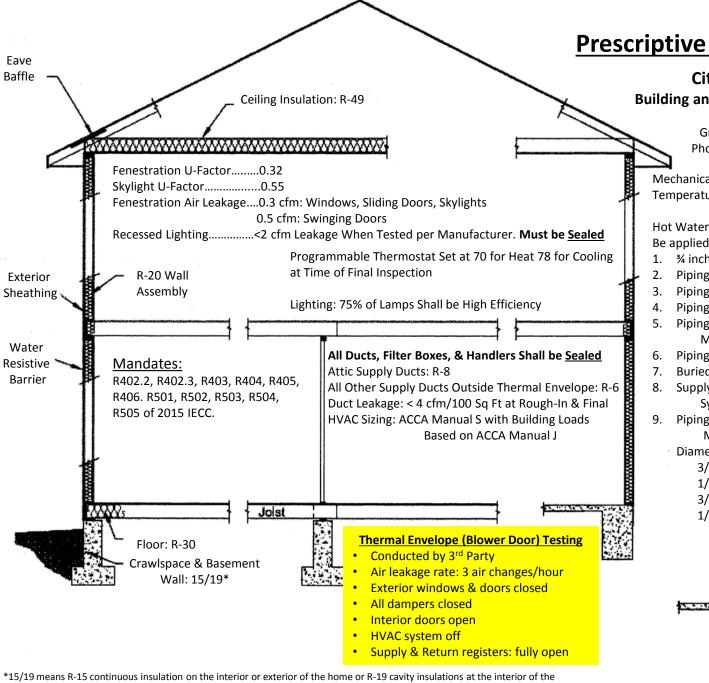
Basement wall. 15/19 shall be permitted to be met with R-13 cavity insulation on the interior and R-5 continuous insulation on
